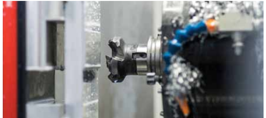
SHAPE's Okuma machines boast 15,000 rpm, 64 tools, and through-the-spindle high pressure coolant.
